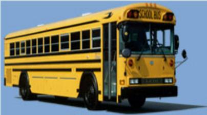
**Type “D”** (“Transit”) school bus means a bus with a body constructed using a stripped chassis. The entrance door is ahead of the front wheels. The bus is also known as a rear engine or front engine transit style school bus.
