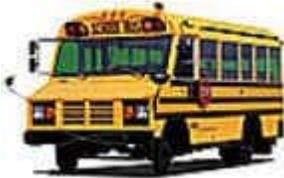
**Type “B”** school bus is constructed utilizing a body on a stripped chassis. The entrance door is behind the front wheels. This definition includes two classifications: Type B1, with a GVWR of 10,000 pounds or less, designed for carrying more than 10 persons and Type B2, with a GVWR greater than 10,000 pounds.
