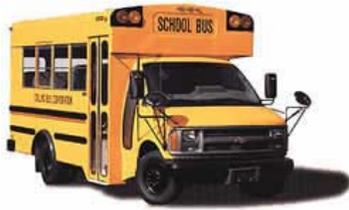
**Type “A”** school bus is a conversion bus constructed utilizing a cutaway front-section vehicle with a left side driver’s door. This definition includes two classifications: Type A1, with Gross Vehicle Weight Rating (GVWR) 14,500 pounds or less; and Type A2 with a GVWR greater than 14,500 pounds and less than or equal to 21,500 pounds.
