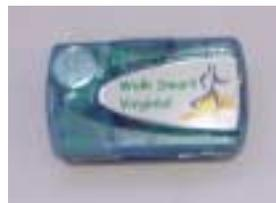
Pedometers fasten to the waist and measure physical activity in a vertical plane—the “up and down” motion of an individual’s hip. Numerous studies have examined the validity of pedometers in assessing the physical activity levels of children and have concluded that the pedometer is a suitable tool for assessing the physical activity patterns of children (Welk, Differding, Thompson, Blair, Dzura, & Hart, 2000).
