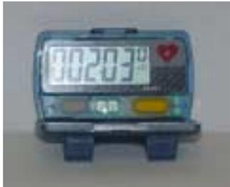
Have them reset the pedometer by holding the button down for about two seconds until the pedometer displays zeros. Resetting the pedometer clears both the steps and activity time counters. The mode button is white and switches the display back and forth between the step counter and the exercise time counter. They can move back and forth between the time and steps mode as often as they like.
