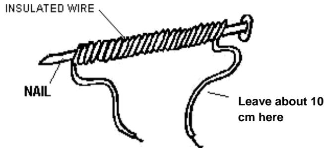
3. After your group has wrapped the wire around the length of the nail, cut the wire so that about 10 cm are left free. Now, use scissors to strip the insulation from the last 2 cm of the wire.
